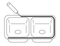
**8.** Position and align sink over the countertop opening and press sink
