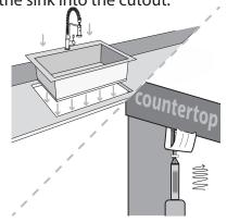
**7b** Tighten the bracket screws until sink is tight to the countertop
