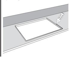
**7a** Bend the clips back and place the sink into the cutout.
