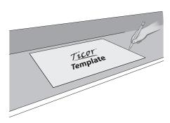
**3** Make cut in countertop, verify hole size, drop sink in and ensure sufficient room for brackets
