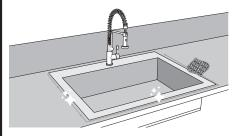
**9** Make the drain connections and attach water supply. Run water into the sink and check for leaks.
