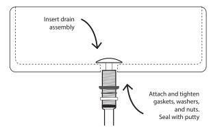
2. Attach the pop-up drain to the sink. Ensure all parts are fully tightened and use plumber's putty on the gaskets to prevent any leakage.
