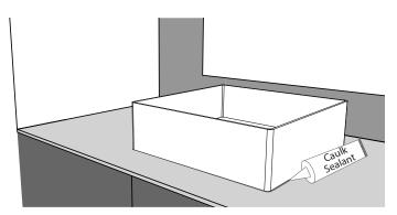
4. Install the sink and connect the P-Trap to the drain. Apply caulking around the base of the sink so there are no gaps between sink and countertop. After the adhesive is dried (refer to adhesive instructions), turn on the faucet for a few minutes and observe to ensure there are no leaks.
