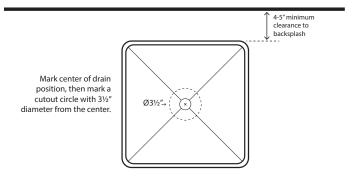
1. Determine the placement of your sink. Ensure at least 4-5" clearance from the backsplash for faucet installation. Mark the center of the drain hole then set the sink aside. Draw a 3½" diameter circle around the center of the drain hole, then cut out this opening.
