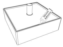
3. Position the vessel sink on the opening of the countertop and double check level and fit. You can use plumber's putty to level the sink if necessary. Remove the sink and turn it upside-down and apply silicone adhesive around the bottom rim of the sink.
